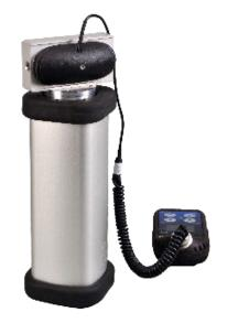
4) Enable Calibration menu in SV 103 by holding Right Arrow button. Select the System check and axis.
