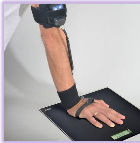
Figure 4-7 Using a bathroom scale as reference level for the contact force check
