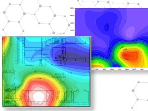
This dust migration map shows the extent of a known primary dust source (lower center) and identified an unknown secondary source in a welding cell (upper left).
