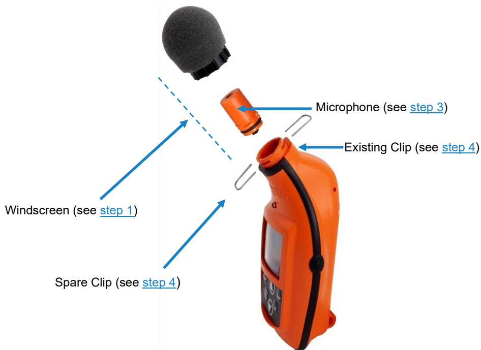
Figure 6-1: Microphone and windscreen assembly
