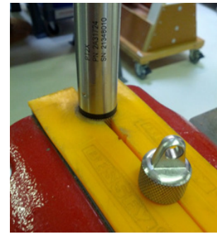
Cableless Sensor—gripping on knurled area
