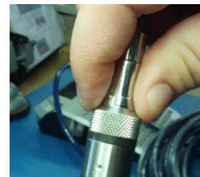
Properly completed—black ring uncompressed
