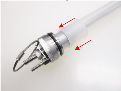
Figure 4-14a: Compression Ring on Bladder
