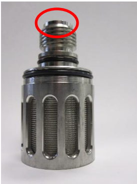
Figure 4-7a: Check Ball Retainer
