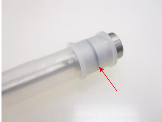
Figure 4-15: Bottom Compression ring with visible O-ring
