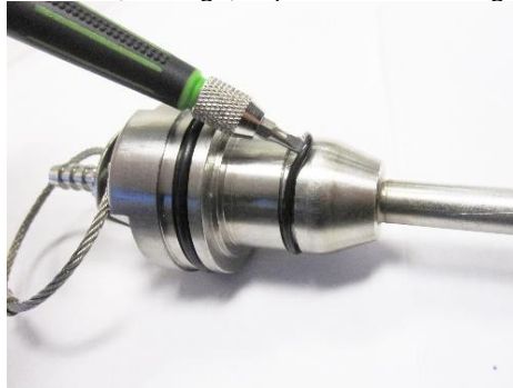
Figure 4-5: Removal of O-rings
