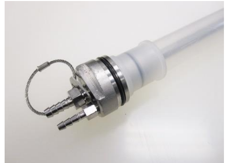
Figure 4-14b: Compression ring secured
