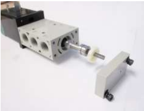
Figure 4-2: Removing Solenoid Parts
