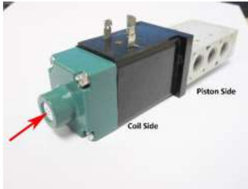
Figure 4-4: Silver button on solenoid
