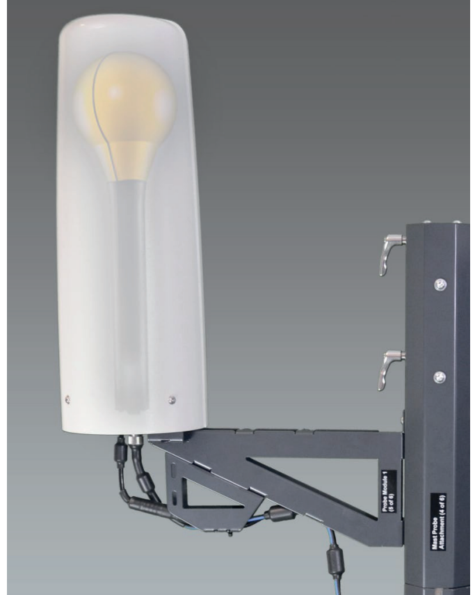
Fig. 2. Probe Module: Isotropic three axis EMF antenna in a radome, with antenna arm for mounting.
