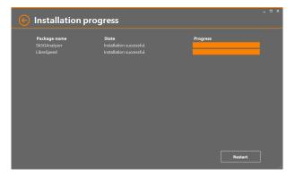
At the end of the installation, click on the 'Restart' button to reboot SignalShark.
