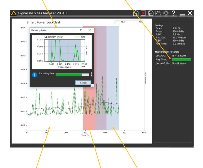
Indicates averaging time related to zero. From this time on, the purple trace shows valid data based on the moving average. Red window indicates automatically determined measured maximum average; level indicated by 'Lev. AVG MAX'
