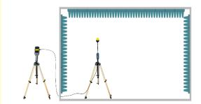
The compact design and handy shape of the Digital Broadband Probe Repeater can also be used as a probe extension, making it much easier to measure in areas that are difficult to access. Even when searching for specific fields, this solution allows you to maintain an overview at all times without losing focus of the FieldMan display.
