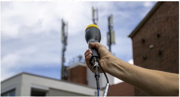
2. Omnidirectional antenna: Pointing it vertically into the sky
