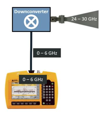
It's down converting mm-Waves into mid-frequency range so that the signal can be more easily transported and processed.
