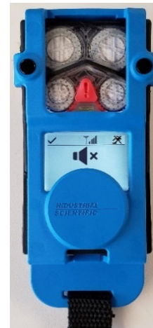
Ventis Pro with Standby Clip (man down and gas readings on standby)
