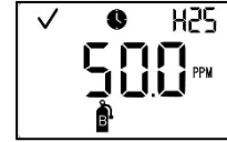
Bump test apply gas
