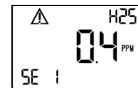
Single sensor data failure
