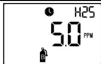
Bump test in progress
