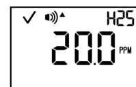
High alarm setpoint
