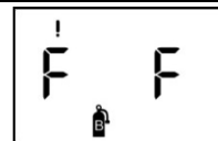
Bump test results (fail)
