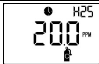
Calibration in progress
