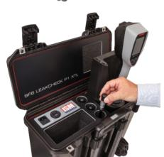
5. Attach the P1 SmartSensor into the plug at the handgun before you switch the instrument on.
