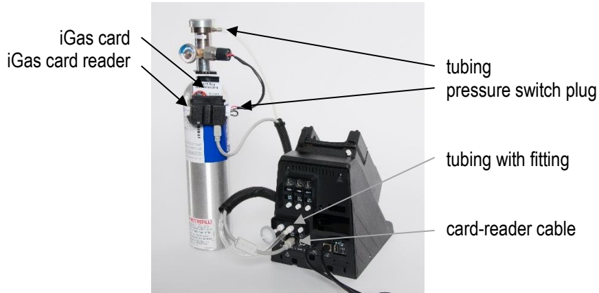
Figure 4-3. iGas Cylinder connected to DSX-L
