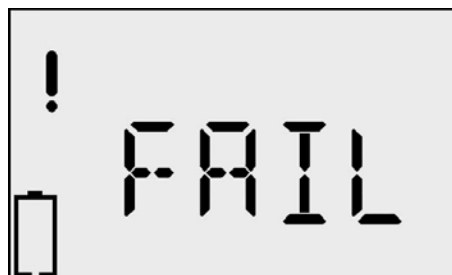
Battery Failure Screen
