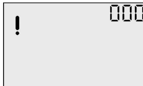
Sensor Missing Error Screen
