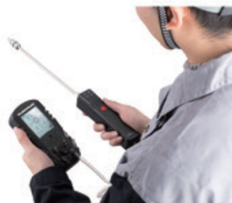
external pump gas detector
