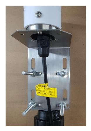
2. Remove the bolts from the top of the mounting assembly. Place the weather station with the plug unattached on the mounting bracket. Ensure the holes are aligned and reinstall the bolts through the weather station.
