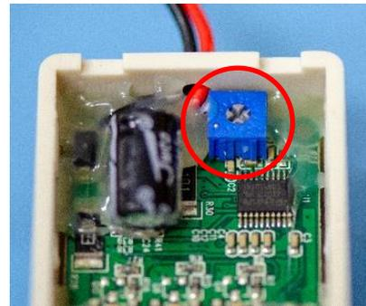
Figure 6-18 – Pump Control Internal
