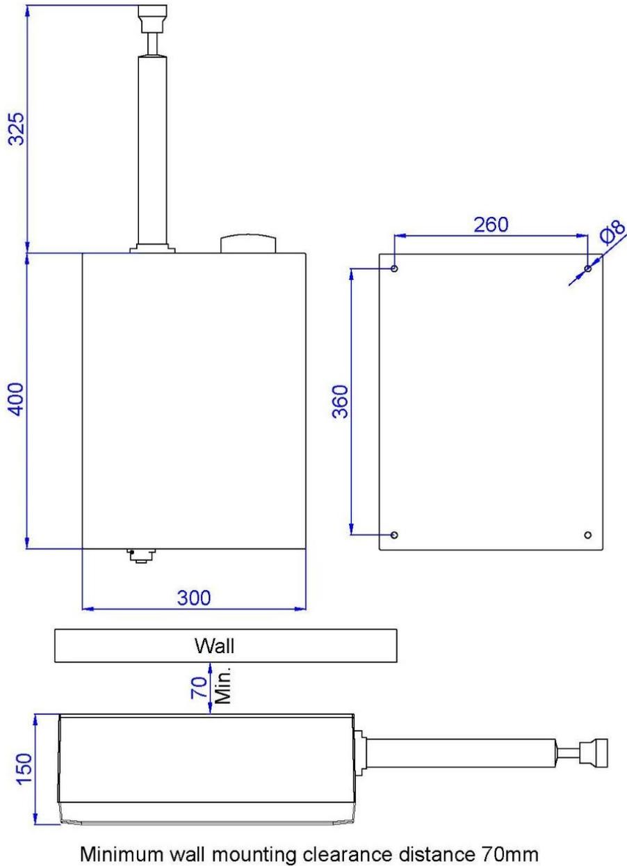
Figure 4-3 – External and Mounting-Point Dimensions (mm)
