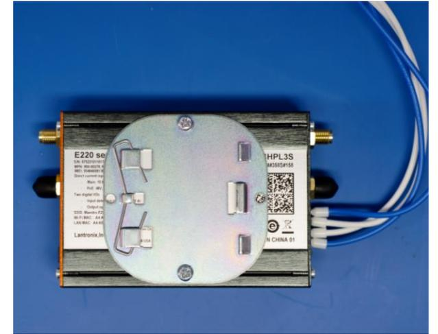
2. Remove the black cover and screw the Wi-Fi antenna into place. Install an ethernet cable between your computer and the LAN1 port of the modem. If you previously turned the instrument off, turn it back on now. Once the blue Wi-Fi LED displays on the modem, it will be ready to configure.
