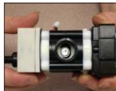
Incorrect: Eccentric off-center and binding yoke
