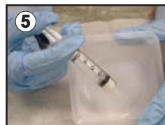
Depress plunger, collect liquid in tray.
