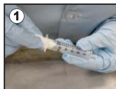
Insert gauze into syringe.
