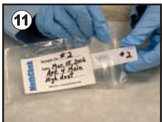
ID sample cartridge. Transport or store in mini bag.
