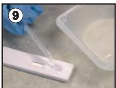
Pipette 3 drops of liquid into "S" well on cartridge.
