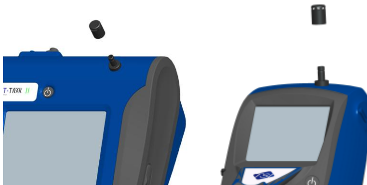
Figure 2-6: Putting on Inlet Cap
