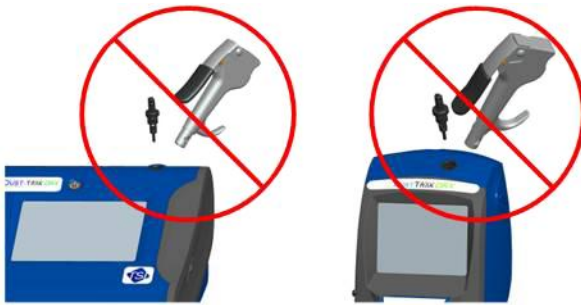
Figure 4-3: Do NOT Blow into Instrument
