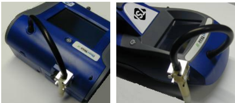
Figure 2-8: Installing Door-Oliver Cyclone
