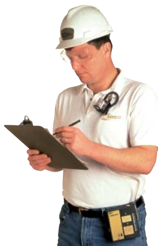
Clip sampling medium to worker and pump to belt.
