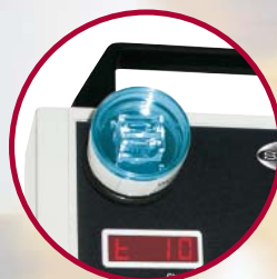
Mount a spore trap cassette directly on pump inlet
