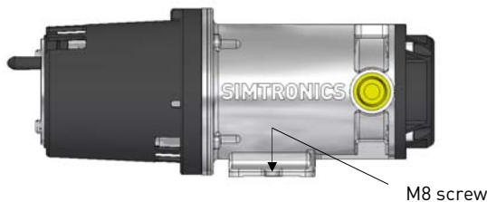
Figure 3.1 GD10P mounted by means of mounting feet
