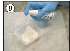
Spray 2 times with Step 2 Developer.
