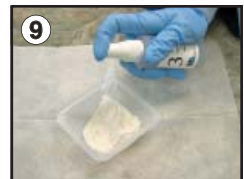
Spray 4 times with Step 3 Developer.
