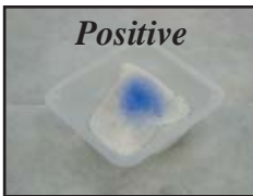
Positive – bright blue color bloom Meth residue detected between 15 and 5000 \mu\text{g} (See Quick Guide for color.)
