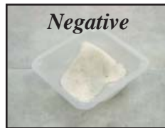
Negative – no blue color bloom Meth residue not detected at 15 \mu\text{g} lower limit of visual identification
