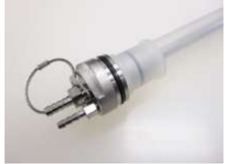
Figure 4-14b: Compression ring secured
