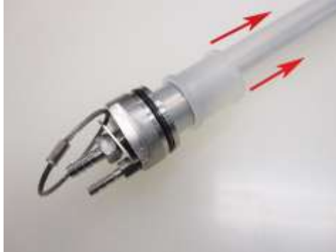
Figure 4-3: Removal of upper HDPE Compression Ring
