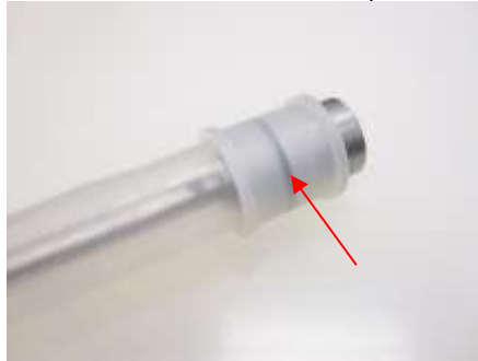
Figure 4-15: Bottom Compression ring with visible O-ring
