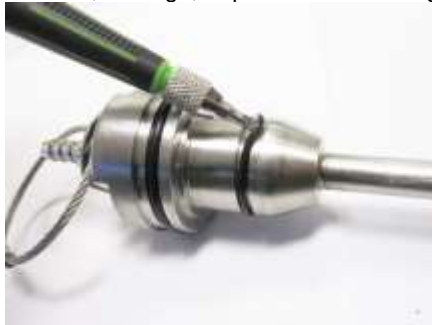
Figure 4-5: Removal of O-rings
