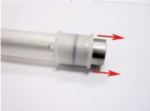
Figure 4-2: Removal of bottom HDPE Compression Ring
