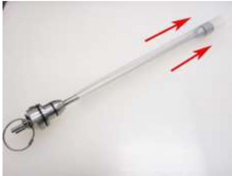
Figure 4-4: Removal of Bladder
