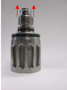
Figure 4-7b: Removing Check Ball Retainer
