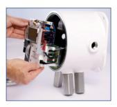
Titan is designed to be easily installed and serviced. Its modular design allows the Ex d case to be installed well in advance of commissioning. The service module can be removed and replaced as a remotely serviceable plug-and-play cartridge.
