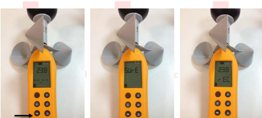
3. The frequency of data recording is based on the sample rate configured by TWLIT. For example, a sampling rate of 10 min means that every 10 min, the device records data once, i.e., 6 readings in an hour. *Please note that every rEC lasts for 120 sec and the data recorded are the average of the 120 sec. When IdLE shows, that means the device is not recording.*
