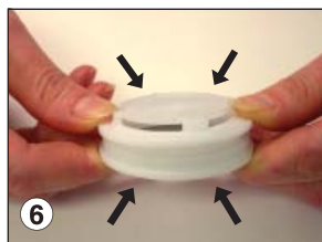
6 Press the filter cassette top into the filter cassette bottom.
