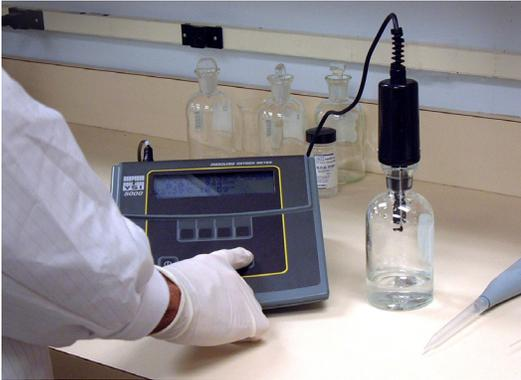
Ease of use, data integrity, expanded range, enhanced digital capabilities - the YSI 5000 Series is engineered to meet the need of highly accurate, reliable dissolved oxygen measurements, primarily to determine BOD but also Oxygen Uptake Rate (OUR) and Specific Oxygen Uptake Rate (SOUR).
