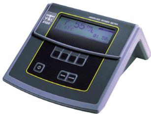
YSI 5000/5100 with the 5010 self-stirring BOD probe simplifies BOD testing. Auto-cal feature on the instruments makes calibration possible with the press of one button.
