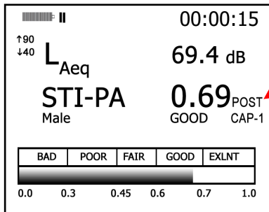
Figure 6-27: Post CAP-1 applied during STI-PA test
