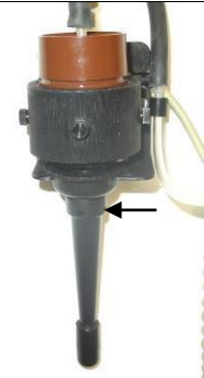
Figure 3.3. Component identifications from left to right: SKC GS-Cyclone for Respirable sampling, GSA-204 adapter, sensor head, filter cassette, and air intake tubing. *Requires the GSA-204 Cyclone adapter to fit.
