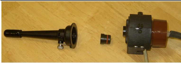
Figure 3.3. Component identifications from left to right: SKC GS-Cyclone for Respirable sampling, GSA-204 adapter, sensor head, filter cassette, and air intake tubing. *Requires the GSA-204 Cyclone adapter to fit.
