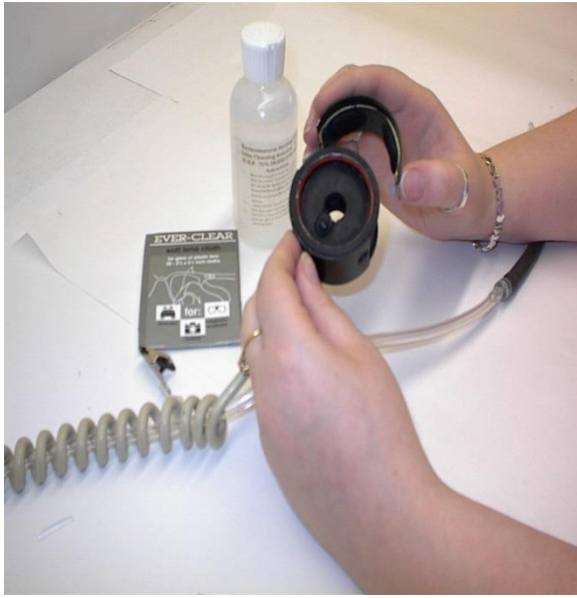
Cleaning the Sensor Optics, Continued Figure 5-4. Dust being removed with low
