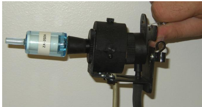
Figure 3.7b. Zeroing filter (p/n ZA-202A) being attached to the Inhalable sampling inlet.
