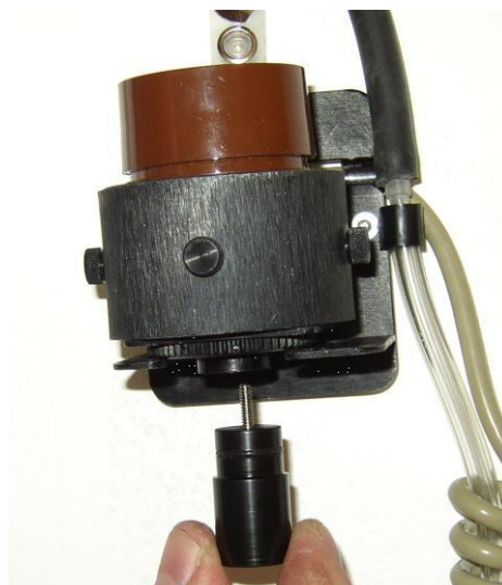
Figure 5-1. Figure of the SM-4000 sensor showing the calibration reference being inserted.
