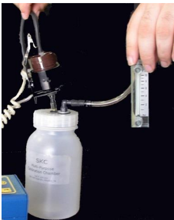
Figure 5-3. SM-4000 sensor connected to CH-103 calibration chamber.
