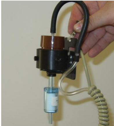
Figure 3.7c. Zeroing filter (p/n ZF-102) being attached to GSA-204 GS-Cyclone adapter.
