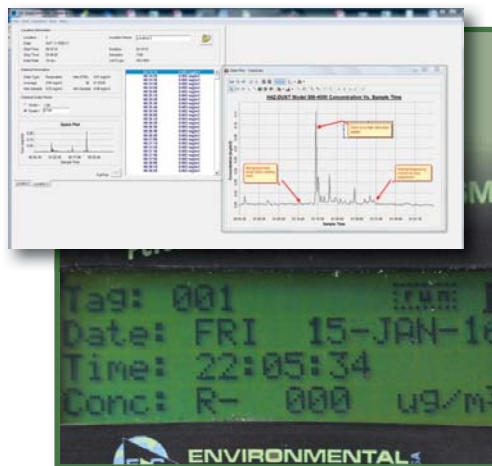
Read dust concentration on the SM-4000 display. Download data for graphing/reporting.
