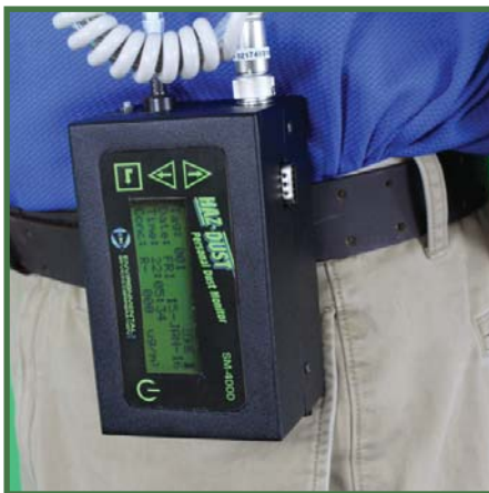
Clip the SM-4000 to a worker's belt.
