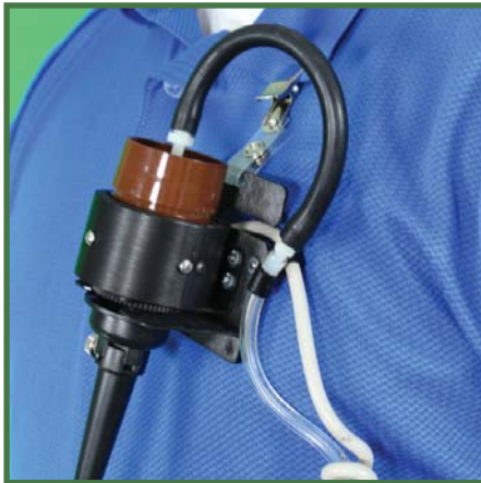
Clip the sensor with GS-3 Cyclone to a worker's collar in the breathing zone.
